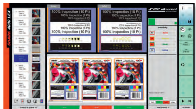
SHARK LEX repeat and defect overview
