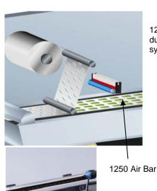
1250 Air Bar blowing dust into a collection system
