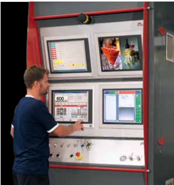
The operator control panel can be enclosed in the press rear frame structure or on a separate console.
