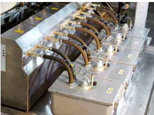
The new pneumatically loaded chamber doctor blade permits toolless end seals and doctor blades replacement.
