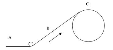
Position (C) is the best position for 801 Anti-Static Tinsel or 850 Anti-Static Cord. Draped over the reel so that it will not get caught in the winding process you can achieve a 90-95% reduction in charge.
