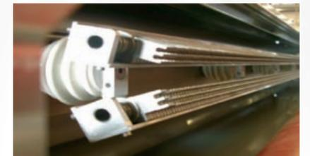
2 x 3-fingered segments enable a perfect Corona discharge at any generator power and speed.
