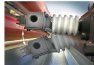
The electrode assembly swings out of harm's way should a large impediment pass through the spray-gap.
