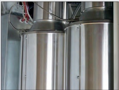
Two molecular sieves towers, high production, made of stainless steel and insulated
