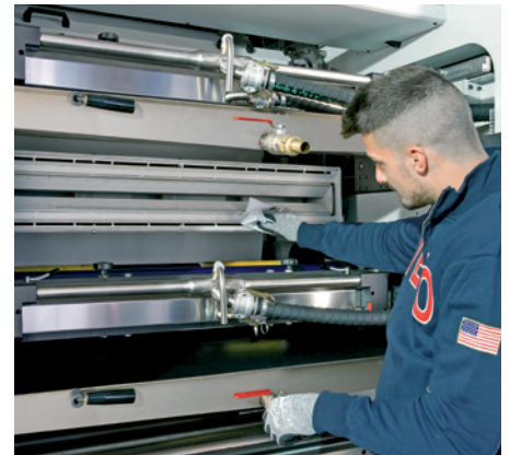
Rotation of the drying box for easy cleaning of the air blades
