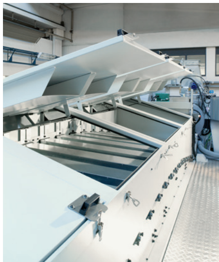
Air blades removal in the drying tunnel for an easy cleaning
