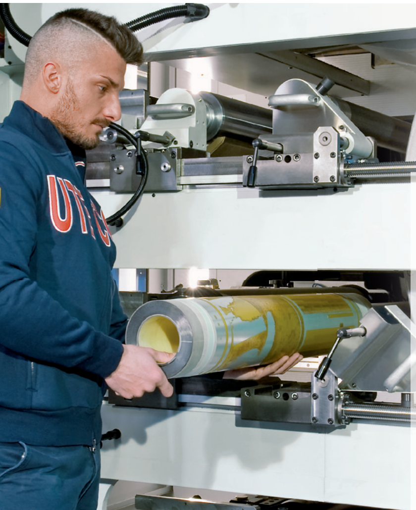
Plate sleeve ejection for fast sleeve change
