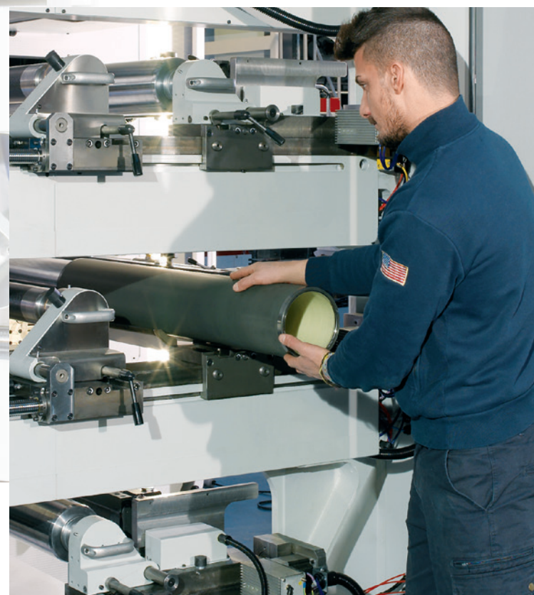
Anilox sleeve ejection for fast sleeve change
