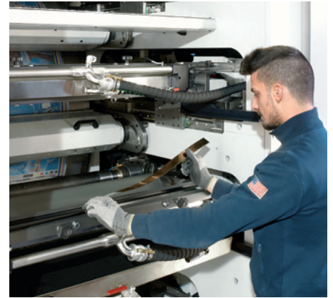
The blade and end-seals change can be performed on-press without tools
